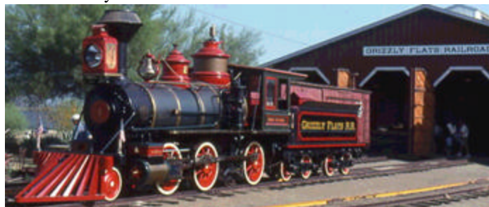
Named for an 1800's opera star, the "Emma Nevada", an 1881 Baldwin 'Mogul' 2-6-0, was the pride of Ward and Betty Kimball's backyard Grizzly Flats Railroad.
